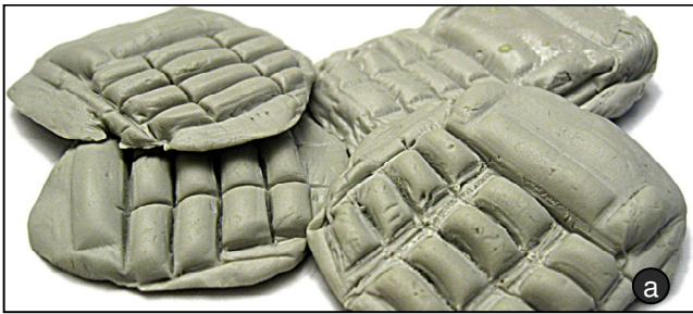
Figure 7. The clay prototypes we used to determine minimum button spacing
